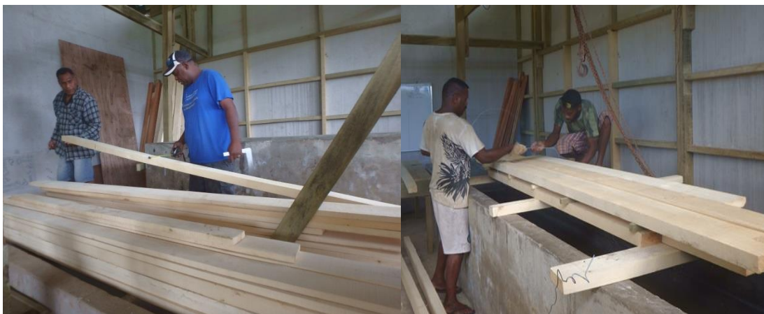
Figure 15: Envelope treatment of first grade timber with Borax at TRF
