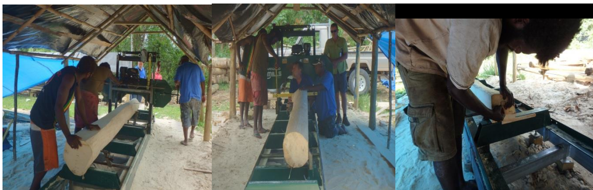
Figure 13: Marking the levelling the logs on the sawmill rail before processing
