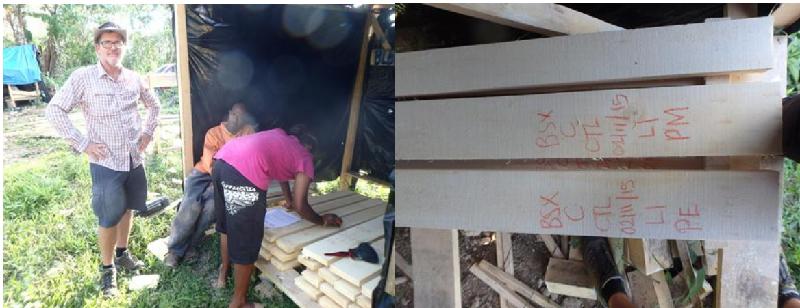
Figure 5: Weighing and recording the weight of the boards
