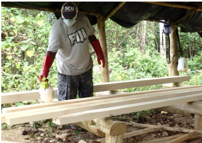
Figure 14: Praying of first grade clear timber with mixture of Taratek and Tanamix
