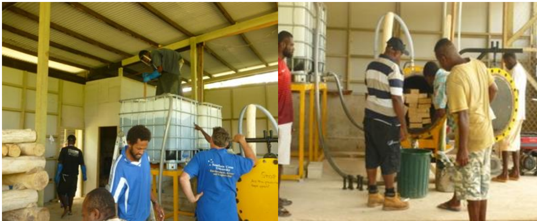
Figure 15 Pressure treatment of structural timber with copper azole preservatives
